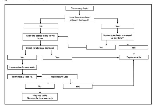
It is important that the cable is checked for physical damage, checks should be made to ensure that no changes have occurred in the physical dimensions of the cable.
